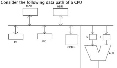
The, ALU, the bus and all the registers in the data path are of identical size. All operations including incrementation of the PC and the GPRs are to be carried out in the ALU. Two clock cycle are needed for memory read operation – the first one for loading address in the MAR and the next one for loading data from the memory but into the MDR.
